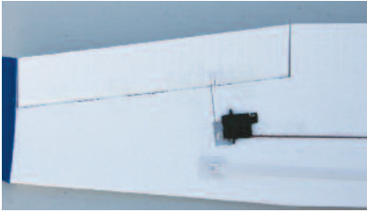
Individual servos are used for aileron control, thus eliminating the often flexible and troublesome linkage employed when using a single servo to operate both ailerons.
