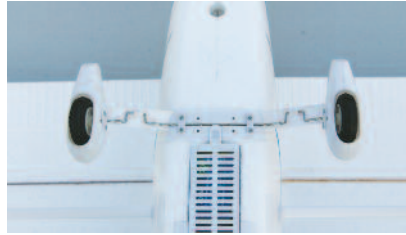
The main landing gear is securely attached to the fuselage yet is rather flexible so the occasional bounced landing won't cause any damage to the aircraft structure.
