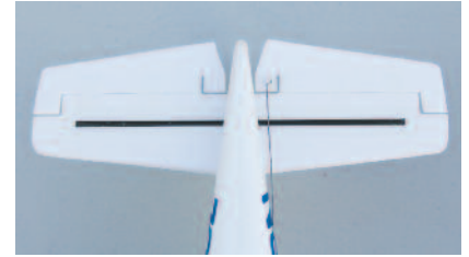
A single carbon fiber rod, which acts as a stiffening spar, is recessed into the horizontal stabilizer and provides considerable strength without adding any perceivable weight.
