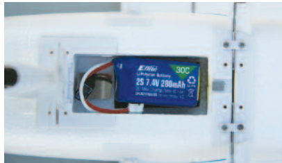
Although snug, the battery compartment is well ventilated and after a number of test flights there was absolutely no evidence of any overheating of the flight battery.
