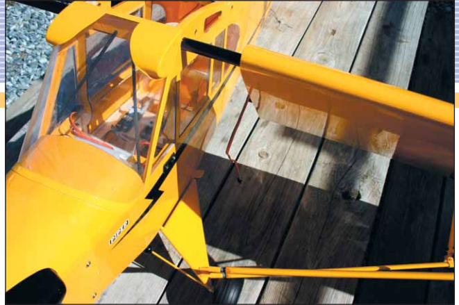
Wings secure over an aluminum joiner, retained by functional wing strut fittings and a nylon bolt through each root rib.
