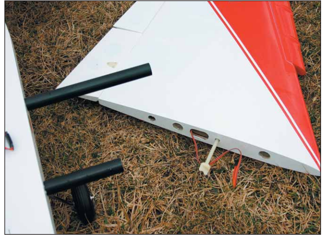
Wing panels mount over two sturdy aluminum tubes. Each one secures with a 1/4-20 nylon "ear" bolt — no tools required.
