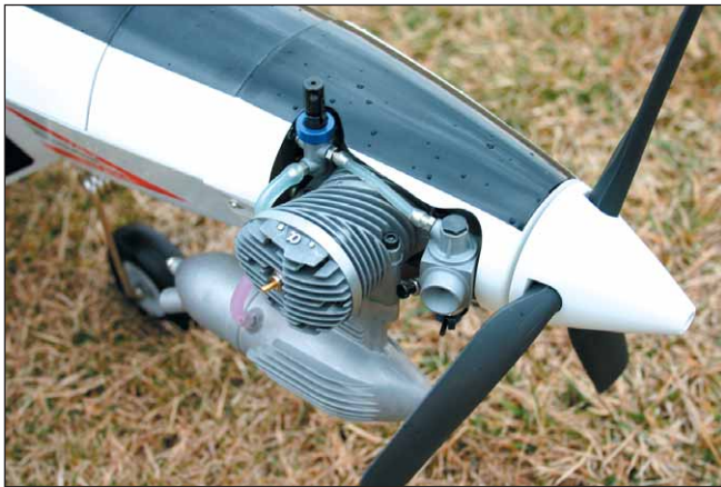
Evolution .46 two-stroke engine is part of TPS (Trainer Power System) package. A three-bladed propeller and rugged nylon spinner complete the Raptor's easy starting power system.
