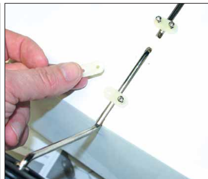
Main gear legs are secured by nylon straps and Phillips-head screws. Nose gear is secured with tiller arm. Assorted hex wrenches are provided in this RTF kit.
