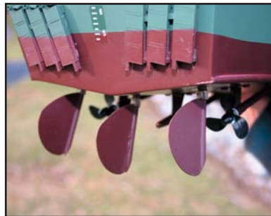
Two massive 550-class, water-cooled, electric motors and a heavy-duty reversing speed control ride inside the PT-109 RC bay. Three rudders and a twin-propeller setup provide turning authority and plenty of planing power.
