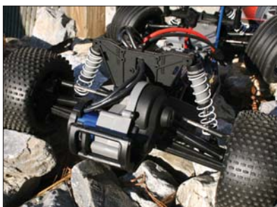
Front- and rear-end chassis views show rugged, composite nylon construction, beefy arms, sturdy coil-over shocks, heavy drive shafts and sealed transmission.
