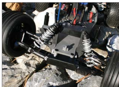
Front- and rear-end chassis views show rugged, composite nylon construction, beefy arms, sturdy coil-over shocks, heavy drive shafts and sealed transmission.
