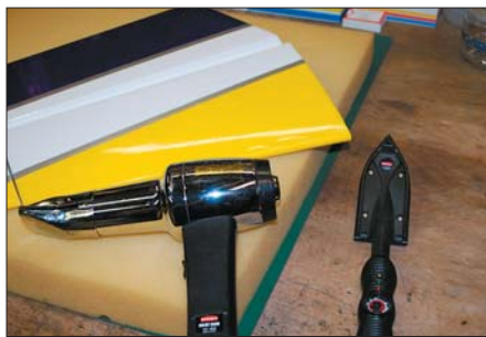
UltraCote covering is expertly applied, with straight color breaks and wrinkle-free corners. Jeff Troy corrects slight blistering from shipping with Hangar 9 covering iron and heat gun. Covering should be ironed down onto all surfaces.
