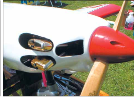
Saito's black powder-coated .82 Golden Knight four-stroke glow engine fits perfectly inside the Harmon Rocket's factory-painted, white fiberglass cowl.
