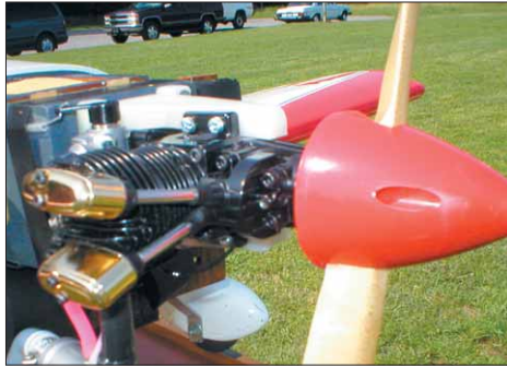
Saito's black powder-coated .82 Golden Knight four-stroke glow engine fits perfectly inside the Harmon Rocket's factory-painted, white fiberglass cowl.
