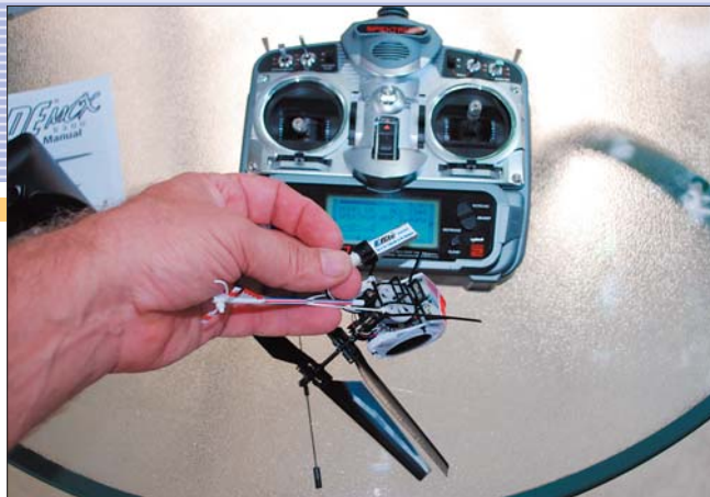
Binding the mCX is easy, and takes roughly 20 seconds. The model should sit level for a 5-second lock-in prior to each flight.
