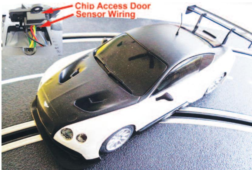
*Sold as an analog car, the Scalextric Bentley is easily converted to digital format by opening the cover located at the front of the chassis and inserting a digital chip that is available separately as an add on sale. When operating in analog mode Scalextric cars will operate on any track, but unfortunately when converted to digital operation Scalextric cars will only operate on Scalextric digital track.*
