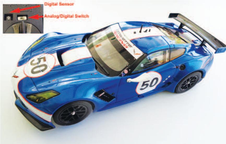
*Carrera uses a slightly different approach as although older cars can be converted to digital, the new cars are digital from the factory, but can be used in analog mode with the flip of a switch. Like Scalextric, when operating in analog Carrera cars will work on any track, but in digital format Carrera cars will only operate on Carrera digital track.*
