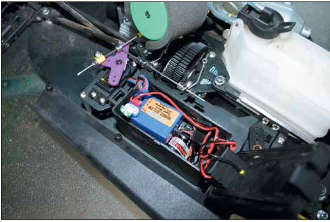
Despite its four-channel capability, Airtronics receiver is able to fit into common two-channel locations.
