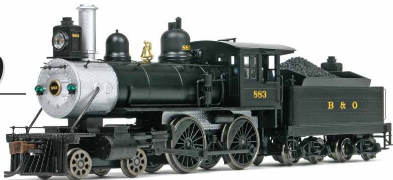
At trackside, the modern 4-4-0 American locomotive is graceful and tall, good for speeds in the 60's and 70's with a light coach load.
