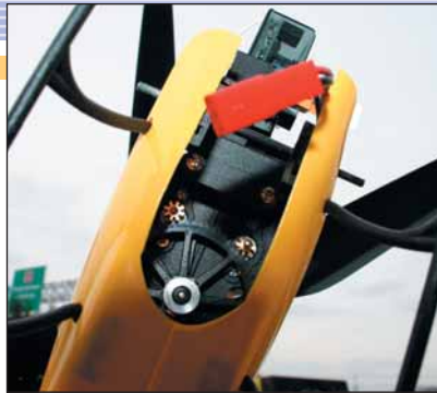
Twin 180 motors and the 4-in-1 FM receiver/mixer/gyro/ESC are factory installed. Lower view shows dual brass pinions and composite main rotor drive gear.
