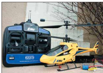
Blade CX helicopter comes with a four-channel RC system, a two-cell lithium-polymer battery and balanced charger.
