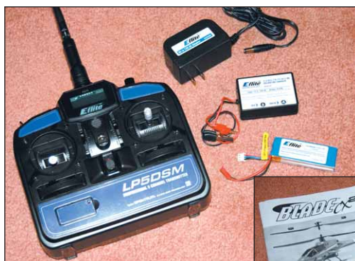
E-flite's Blade CX2 comes with a Spektrum 2.4GHz RC system, an 800mAh LiPo battery and a DC balance charger with an AC adapter. A 48-page manual and an instructional DVD are also included in this full-feature package.
