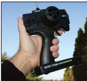
TACTIC brand is a Great Planes exclusive. The pistol-grip transmitter features throttle and steering trims, and the rate knob allows precise adjustments for steering on the fly. The receiver, steering servo and ESC are factory installed.
