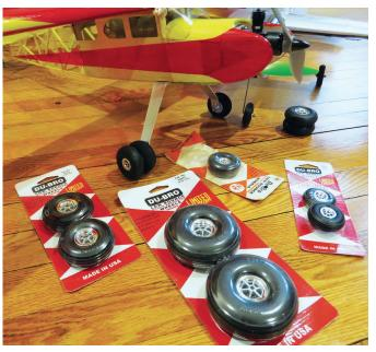
On heavier models, the Du-Bro wheels give a scale squash from the weight. Another advantage is how quiet the low-bounce wheels are on asphalt. Heat-shrink-covered models tend to amplify any wheel noise like a drum. The recently re-released wheels are still outstanding, maintaining the same high quality as from their original release years ago.
