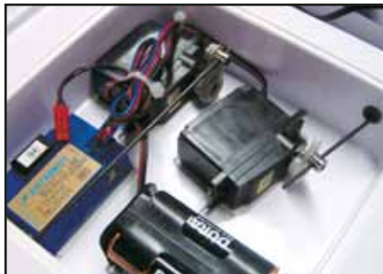
HM's review model uses Airtronics RC with standard servos, all held with supplied double-sided tape.
