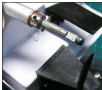
Graham uses Great Planes' Pro Threadlocker (blue) to assure solid retention of drive dog and propeller collar, as well as all rudder fittings and trim tabs.
