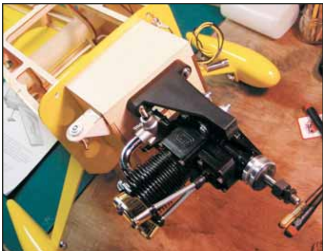
Saito 100 Golden Knight four-stroke, Great Planes' Fuel Filler Valve and Sullivan Products' Remote Glow Plug on the front end.
