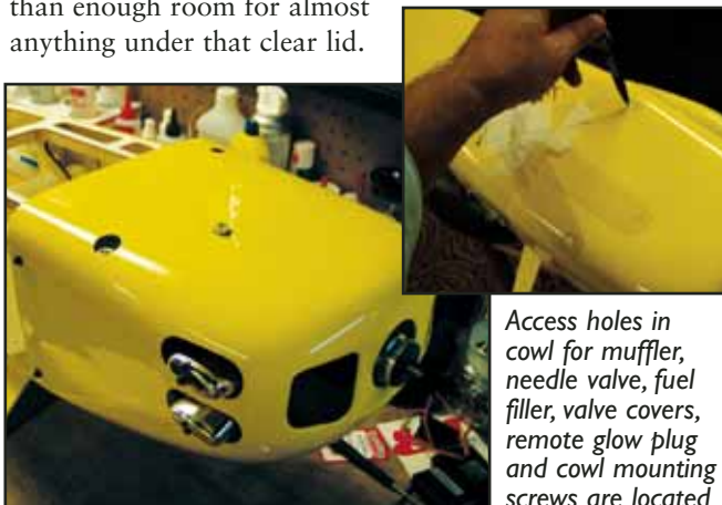
Access holes in cowl for muffler, needle valve, fuel filler, valve covers, remote glow plug and cowl mounting screws are located with clear plastic templates, then marked and cut or drilled to size. Finished cowl is neat, clean and uncluttered.
