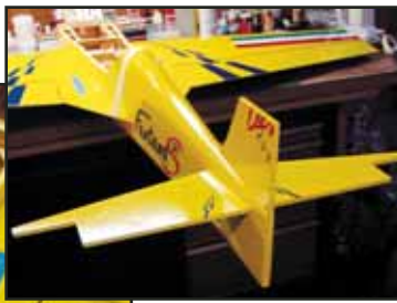
Trailing edge root fillets are secured to the wing panels, then the horizontal stabilizer and the vertical fin are
