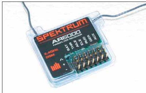
Six-channel Spektrum receiver sports a pair of antennas at a 90-degree angle. TX and RX are always communicating on two frequencies.
