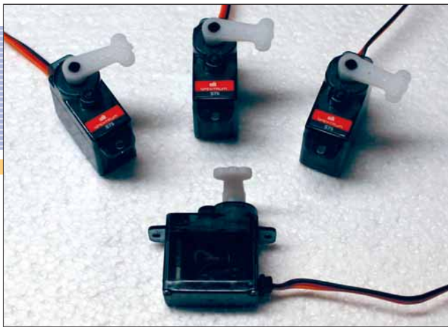
Spektrum S75 Sub-Micro Servos weigh close to 1/4 ounce, and deliver 17.2 oz/in of torque at .12 sec/60 degrees transit time.
