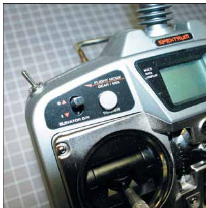
Spektrum six-channel computer transmitter is fully programmable, with dual rate, exponential, mixing options, reversing, digital trims and 10-model memory.
