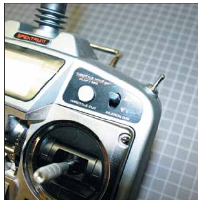
Spektrum six-channel computer transmitter is fully programmable, with dual rate, exponential, mixing options, reversing, digital trims and 10-model memory.
