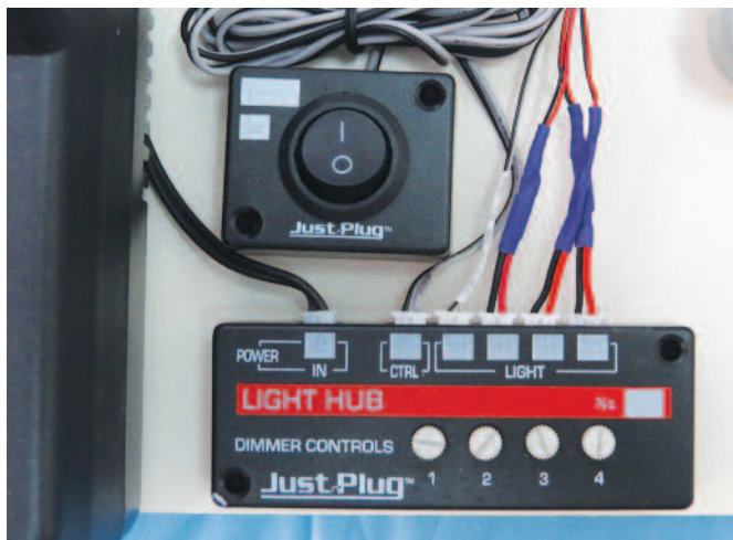
Every manufacturer has gone to great lengths to simplify putting its products into service and Woodland's Just Plug controls all of the layout's lighting to include the different structures and street lights.
