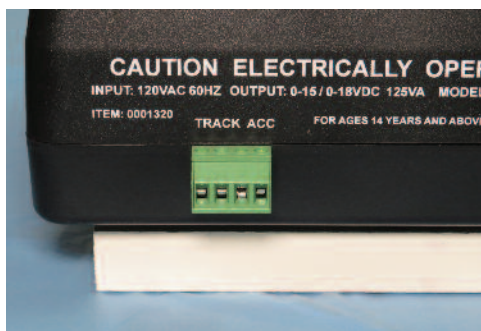
Although digital is the primary control of the layout, there is still a lot of analog used, and to power the outer loop of rails along with the analog accessories, the MRC Throttle Pack 9950 with its simple to incorporate track and accessory power output terminals was selected.
