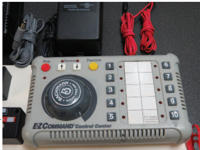
Since the majority of the layout is designed around digital control, selected for use was the Bachmann E-Z Command control center. This little marvel of engineering can control up to nine individual locomotive along with each locomotive's features all at the same time.
