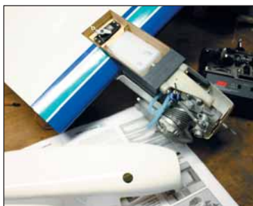
Nacelles and RC bay are designed for effortless radio installation. Engine mounts are included, and come factory installed. Pushrods are also factory installed, and even the fuel tubes and stoppers are assembled and ready to fit into the tank.
