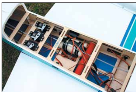
Nacelles and RC bay are designed for effortless radio installation. Engine mounts are included, and come factory installed. Pushrods are also factory installed, and even the fuel tubes and stoppers are assembled and ready to fit into the tank.
