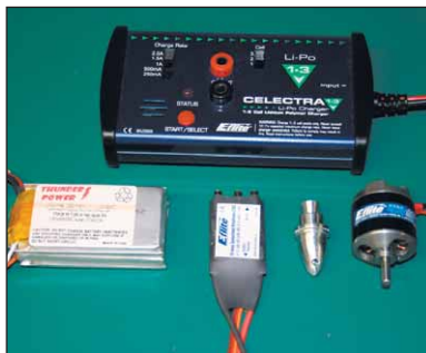
HM's review model uses an E-flite Park 450 Brushless Outrunner Motor, an E-flite 20A ESC and a Thunder Power 3S 1320mAh LiPo battery. RC system selected is the Spektrum DX7 and AR6000 receiver, four E-flite S-75 servos, two 3-inch and two 18-inch extensions.
