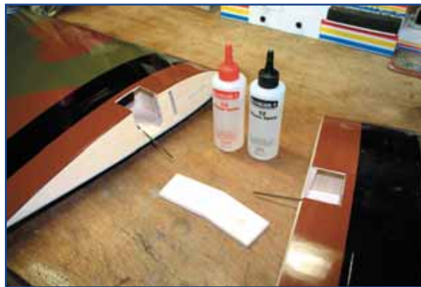
Wing assembly couldn't be simpler. Use Hangar 9 Slow-setting Epoxy to join the panels over a hardwood dihedral brace. Factory joint on HM review model was a perfect fit.
