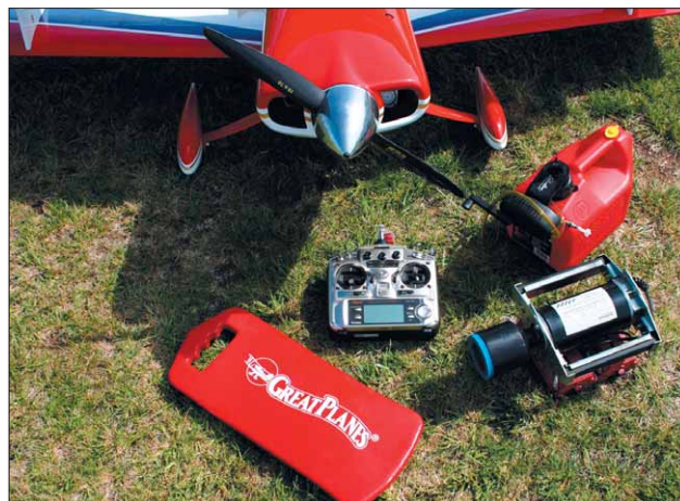
Field support items included Du-Bro gas container with Slimline Products manual gasoline pump, Sullivan Model 4 Mega-Torque electric starter, Futaba 9C transmitter and Great Planes knee pad.
