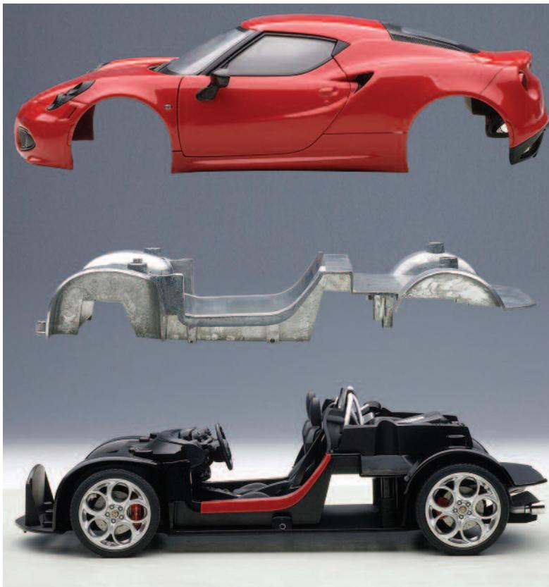
*With AUTOart's composite models, the company pairs a die cast interior with a newly developed injection acrylonitrile butadiene styrene, a thermoplastic polymer with special blend of different materials for reinforcement, utilizing the benefits of both materials to create the highest quality models the company has produced.*
