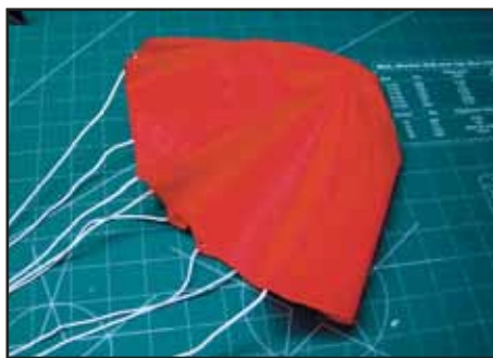
Oracle uses 18-inch Nylon parachute
