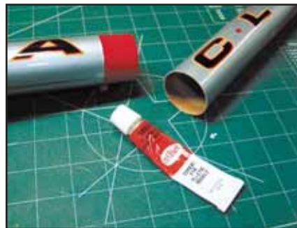
Upper tube is joined to the body with Testor's model cement.
