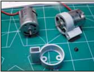
Twin electric motors are fastened to plastic mounts with two screws. Basswood motor sticks in the nacelles carry the completed motor assemblies.
