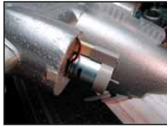
Twin electric motors are fastened to plastic mounts with two screws. Basswood motor sticks in the nacelles carry the completed motor assemblies.
