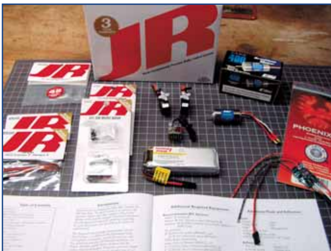
Extras include JR's Airpack Micro, extra 241 sub-micro servos and long servo arm sets, an E-Flite Park 400/4200KV brushless motor, Thunder Power 3-cell Li-Poly battery and a Phoenix-25 brushless/Li-Poly electronic speed control from Castle Creations.
