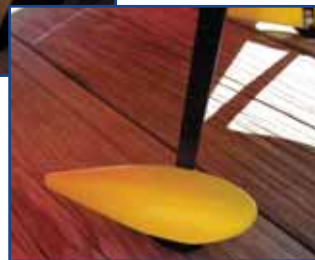
E-Flite's Mini Funtana uses a rugged carbon fiber wing joiner, and the one-piece carbon fiber landing gear provides a sturdy mounting point for the model's painted fiberglass wheel pants.
