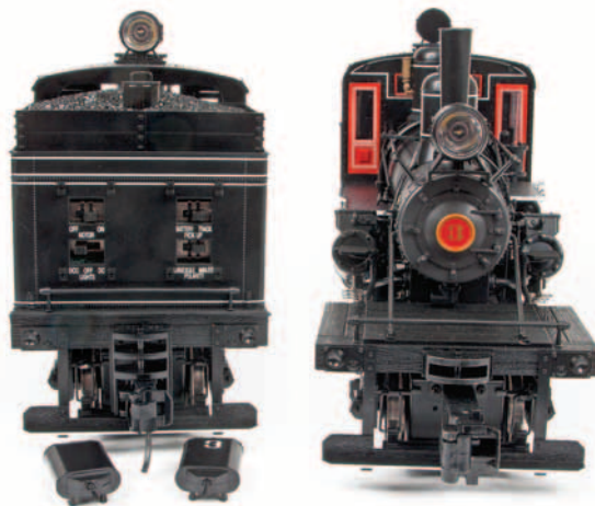
The front and rear views reveal a number of interesting details. Hidden behind the sand tanks are the setting switches for the motor, lights and polarity.
