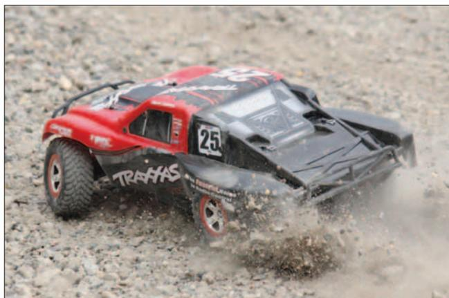
*Nailing the throttle on loose gravel immediately spins the rear wheels, resulting in a shower of debris.*
