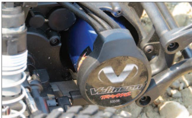
*The Velineon brushless motor applies a whole lot of power to the two-wheel drive chassis.*
