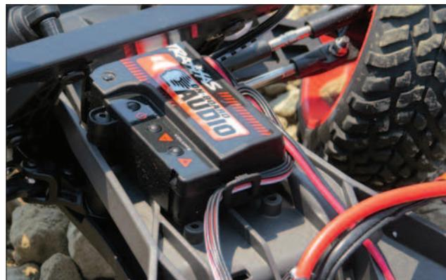
*Adding even more excitement to the package is the OSB module that provides full-scale sound.*
