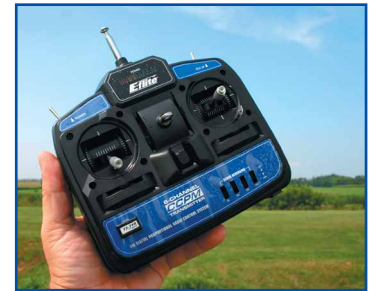
CCPM mixing and idle up are standard features in the Blade CP's six-channel transmitter.
