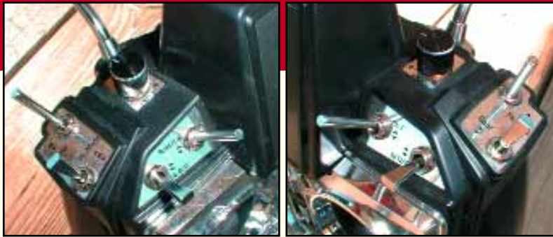
Left-hand transmitter switches include the trainer function, flight mode, dual rates for elevator and rudder, and VR1 for variable flap control and helicopter functions. Right hand switches select flight condition, landing gear, channel 7, dual rates for aileron and VR2 for other variable function controls. Digital trims are easy to use and easy to find.
