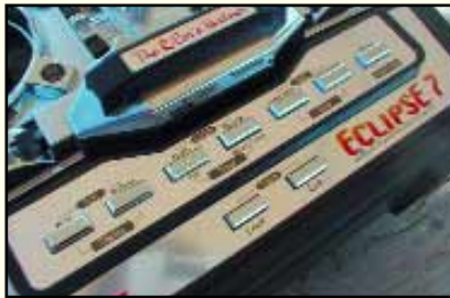
Enter the main menu with the two Edit/Display buttons, then use them to scroll through the trim, dual rate, mixing and other programming features. Use the cursor buttons to select the channel. Data buttons set travel, end point, exponential and more.
