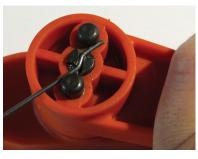
slowly and wait until it's fully cooled before proceeding. This step will remove the temper, making it less prone to breaking.
