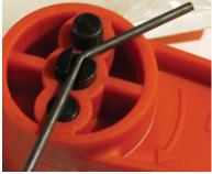
By simply rotating the wire for the next bend and making sure each bend is parallel to the next, you are rewarded with excellent results.
