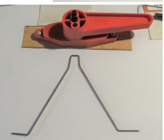
Here's a set of former-mounted main landing gear, completed in a few minutes. I found that if the wire fits a little looser than fully tight, I had better results and less breakage even with the very hard, thin wire. Even with the thicker wire, I was surprised how little effort was required.
